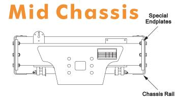
Mount the BT1400H cross member between the inside webs of the chassis rails for high trailer drawbars. **Special Build -** This option needs to be specified when ordering.
