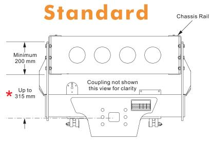
The Standard mounting orientation for the Bartlett BT1400H towbar is slung under the chassis through sideplates externally bolted.
