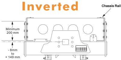
Invert the Bartlett BT1400H towbar to achieve the highest possible centre of coupling height using the standard (shortened) sideplates.
