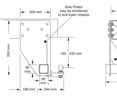
$^{*}$  50 mm Ball, sideplate braces sideplate bolts and holes not included - Shown for illustration only
